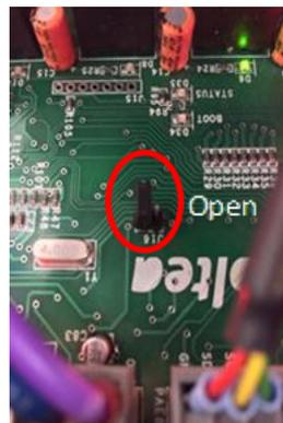
**NOTE:** The jumper on the PCB should be in the open position before connecting to the laptop. Open position is default for the jumper, check only when unable to connect.
