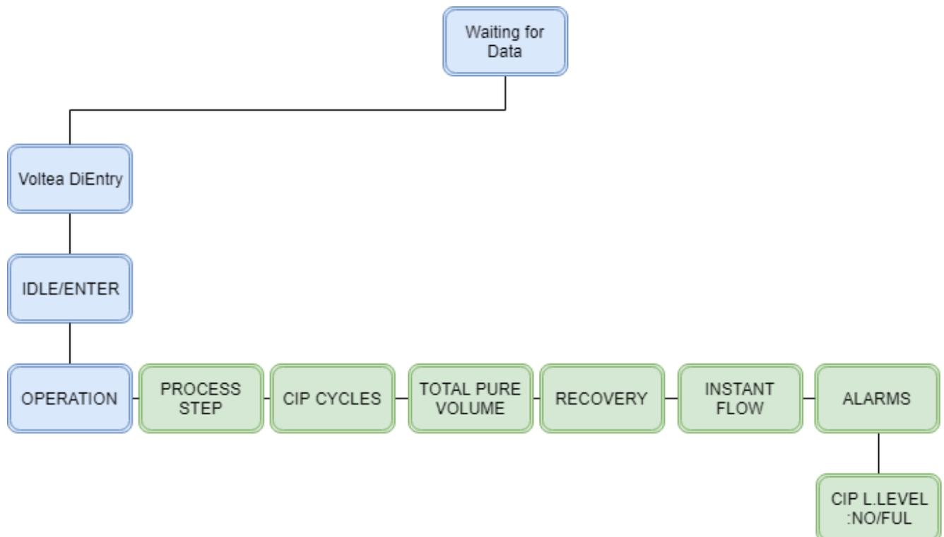
**NOTE :** CIP solution level is calculated based on the CIP's pump capacity to exhaust 3L of CIP solution. For this reason, it is mandatory to reset the CIP alarm once the CIP bottle is refilled. Around 103 ml of CIP solution is used per CIP event.
