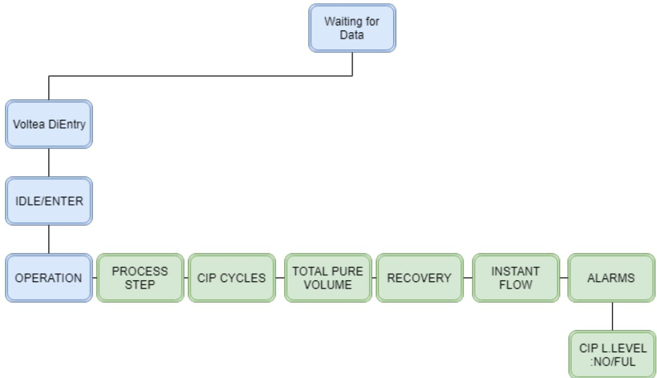
**NOTE:** CIP solution level is calculated based on the CIP's pump capacity to exhaust the 3L of CIP solution. For this reason, it is mandatory to reset the CIP alarm once the CIP bottle is refilled. Around 103 ml of CIP solution is used per CIP event.
