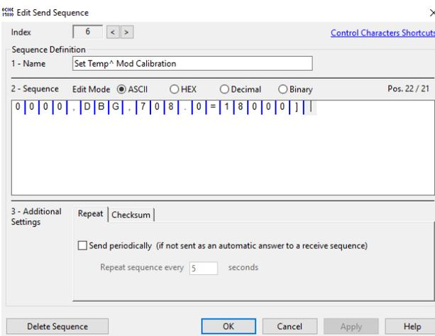
**Note:** If the probe is not at room temperature, wait for 5 minutes for it to reach room temperature before calibrating. Clicking the Read Temp^ Mod Current Temperature will display on screen the probe temperature reading. When this reading is stable the probe reached room temperature.
