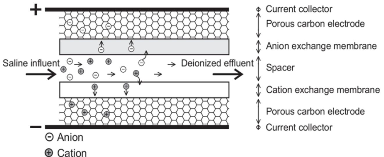
A CapDI module consists of a housing which contains multiple stacks of parallel unit cells. Each unit cell consists of two porous carbon electrodes separated from each other by a spacer. On top of the electrodes, ion exchange membranes are placed. The spacer between the membranes acts as a flow channel to transport the water to be desalinated.
